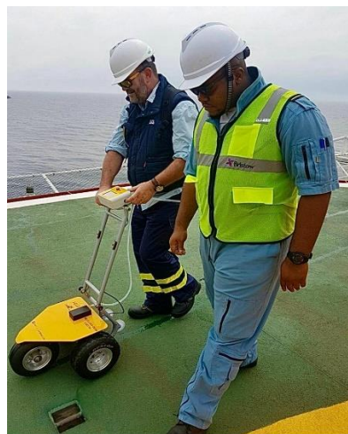
Fig. 3. Helideck inspectors operating the Findley Irvine equipment
