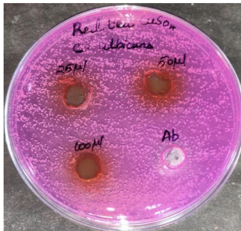
Fig. 3. Zone of inhibition of red tea mediated copper nanoparticles by disk diffusion method showing anticariogenic activity against C. albicans
