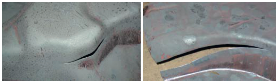
FIGURE 4: Fractures of the A-pillar during hot stamping.
