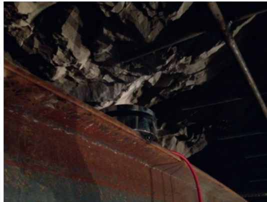
FIGURE 35: Installation diagram of soil pressure sensors.
