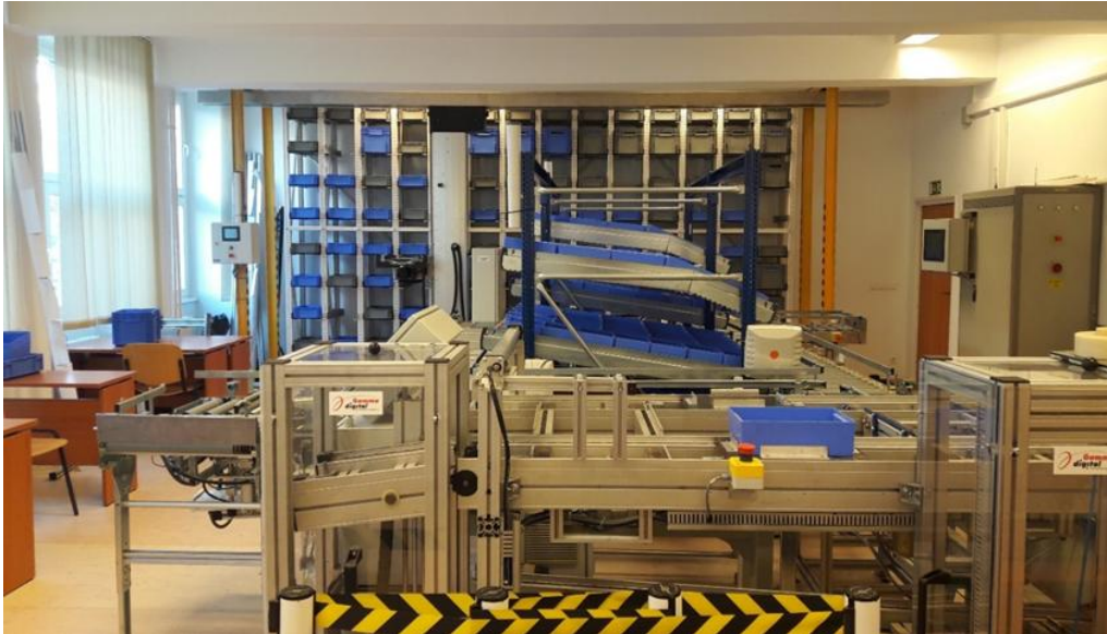
Fig. 1. The general layout of the integrated materials handling system of the laboratory (the palettizing station is in the foreground, while the conveyor track and the automated storage system are in the background)
