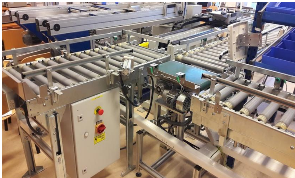
Fig. 2. A turning table with a pneumatic gripper on the left and an RFID reader on the right
