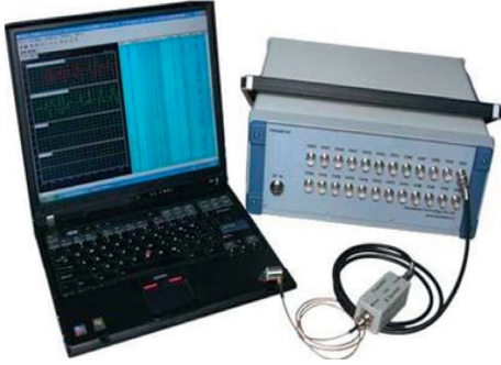
FIGURE 4: SAEU2S multichannel acoustic emission signal measurement system.
