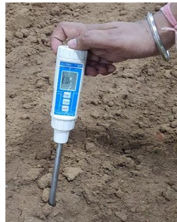
(a) Measurement of soil moisture content in the experimental field
