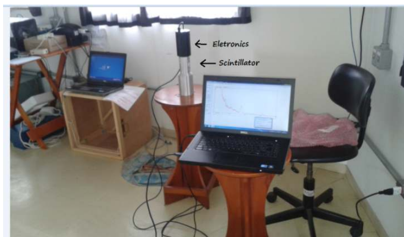
Fig. 1. View of the gamma scintillator associated with electronics and computer
