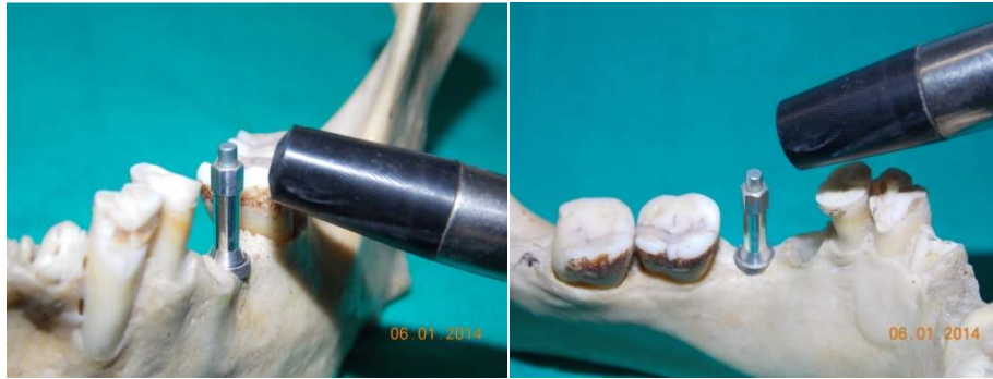
Figs. 7, 8. Showing implant stability measurements made using RFA device in buccolingual and mesiodistal direction
