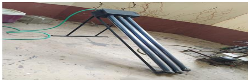
Fig. 20 Evacuated tube collector
