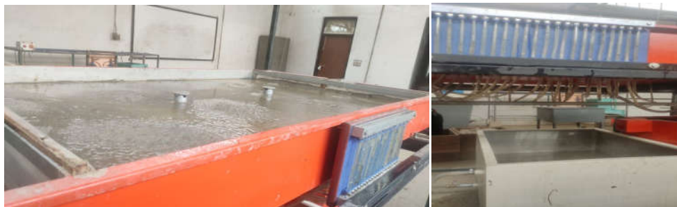
Figs. 5. (a) Aquifer model and pump locations (b) manometers positions and connection with soil plot and well
