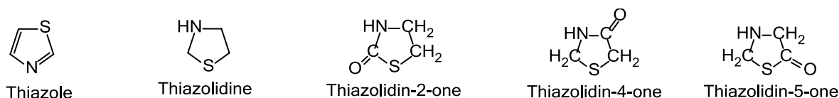
Fig. 4. Ring structures of thiazole and its transformed moieties
