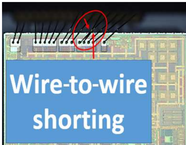
Fig. 1. Wire-to-wire shorting defect
