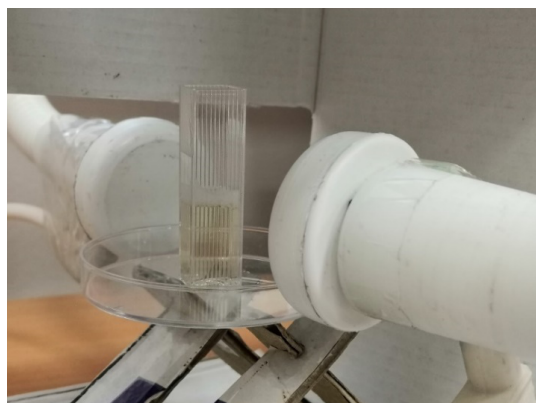
Fig. 3 Installation of a cuvette between the electrodes of the UHF-therapy apparatus.
