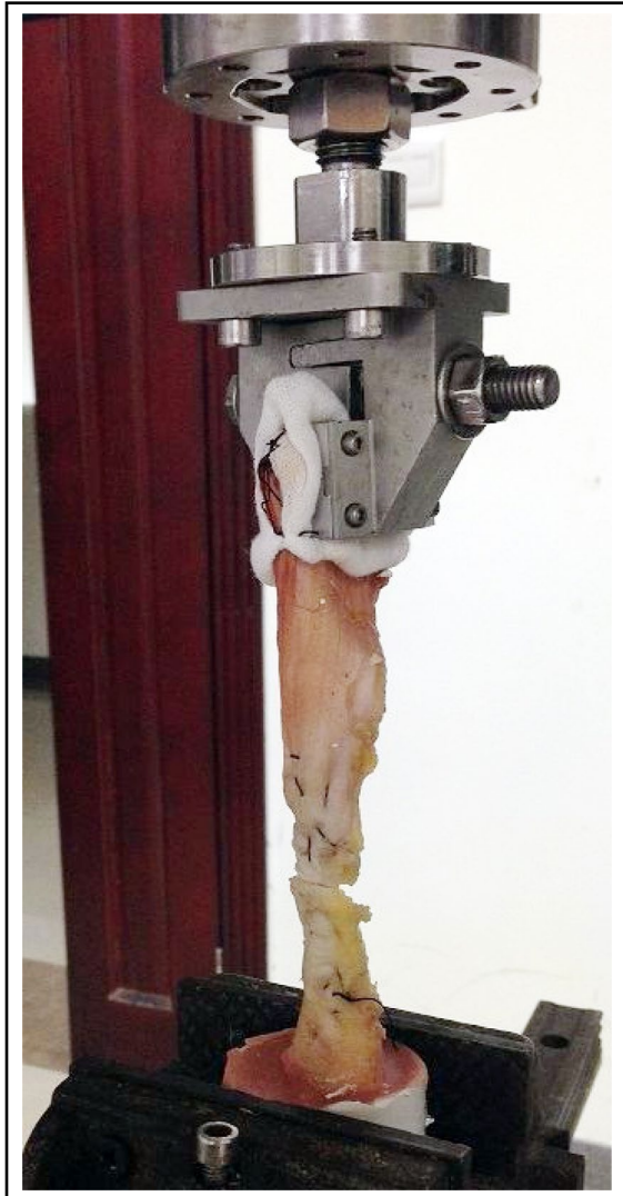
Fig.1: The biomechanical test of rupture of Achilles tendon and repair by different suture techniques.
