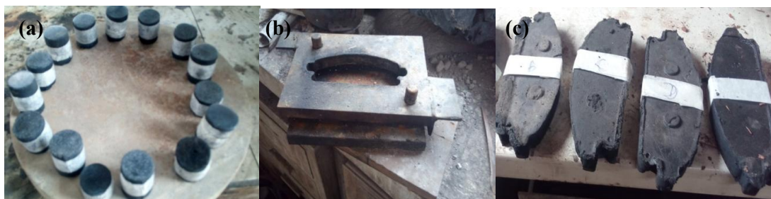
Fig. 2. Composite samples and mold (a) test samples, (b) mild steel mold, (c) brake pad samples
