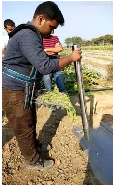
Fig. 4. Planting seedlings on mulch sheet with developed transplanter
