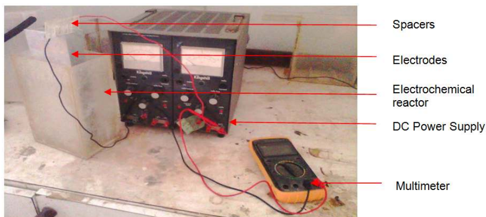
Fig. 2. Laboratory set-up of the batch electrochemical process
