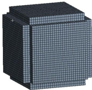
Fig. 8. Mesh grid of the fluid domain in the cancellous microstructure bone. 38,712 nodes, and 35,451 unit numbers
