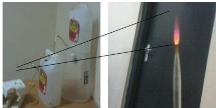
Fig. 4. Biogas burning with a bright flame
