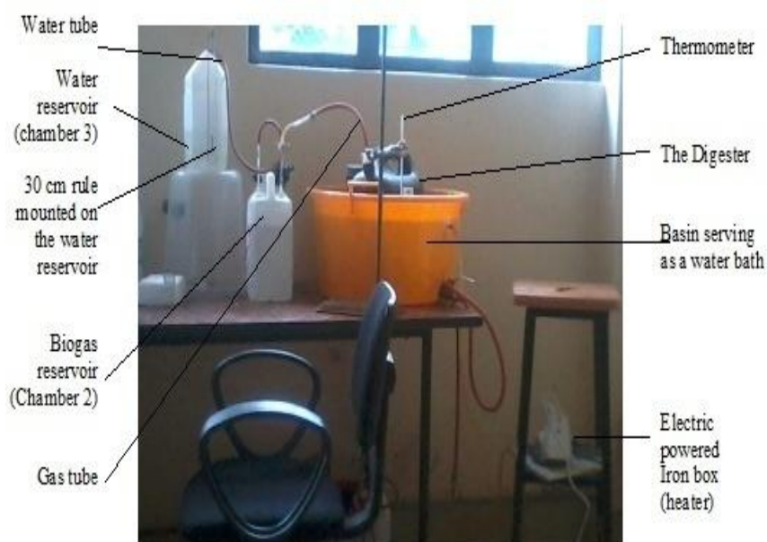
Fig. 9. The setup of the laboratory scale biogas digester system
