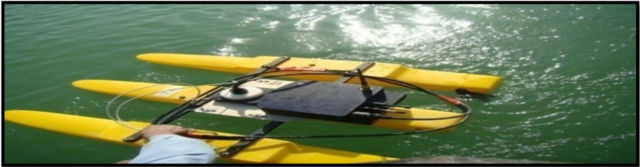
Figure 4. Calculation discharge by ADCP device.
