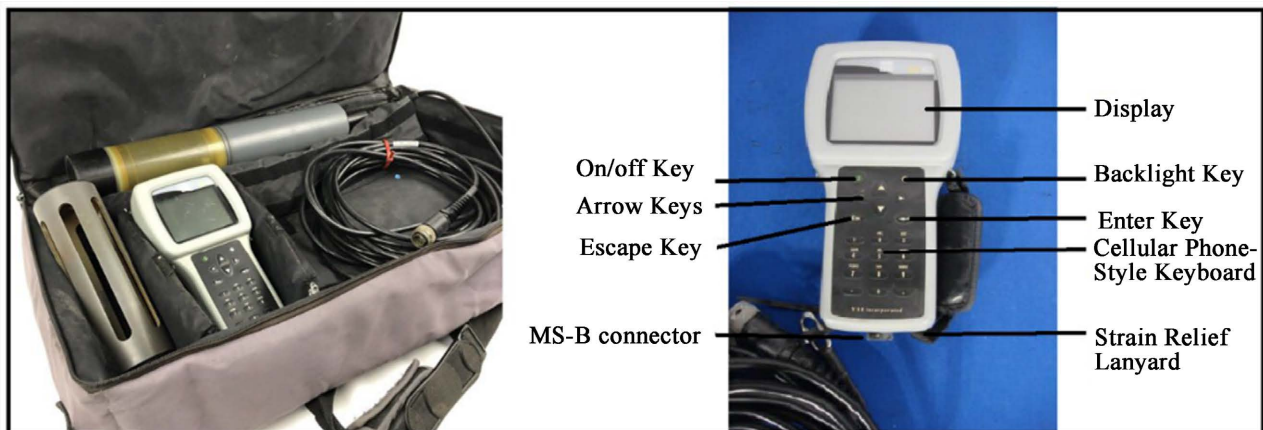
Figure 3. The device YSI incorporating 650 MDS that tested EC, TDS and Te.
